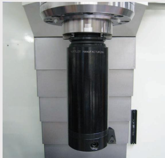
Rottler Boring and Sleeving Cutterhead installed in massive heavy duty EM69ATC Spindle.
