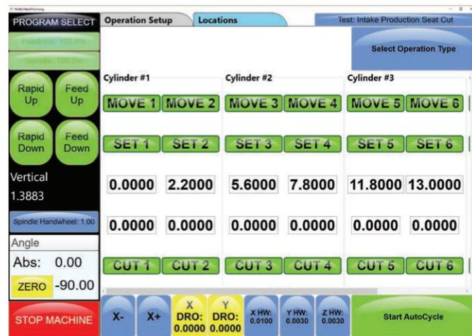
Multiple Cylinders/Valve Guides are programmed so that the SG10XY can move automatically from guide-to-guide – unattended. The slider allows 24 valve guide centers to be programmed in X and Y location.
