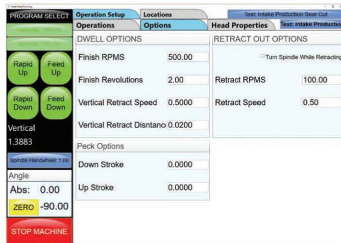
Dwell and Retract are the important settings that allow precision valve seat machining for features such as surface finish and CONCEN.
