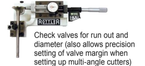
Check valves for run out and diameter (also allows precision setting of valve margin when setting up multi-angle cutters)
