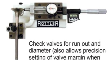
Check valves for run out and diameter (also allows precision setting of valve margin when setting up multi-angle cutters)
