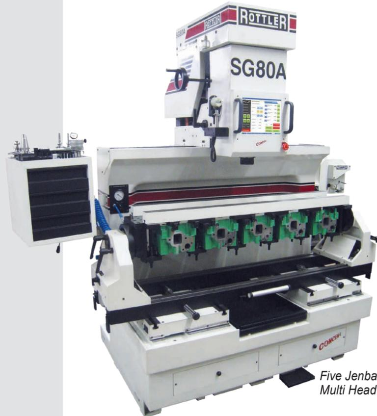
Five Jenbacher cylinder heads set up on special Multi Head 360 Degree Roll Over Fixture
