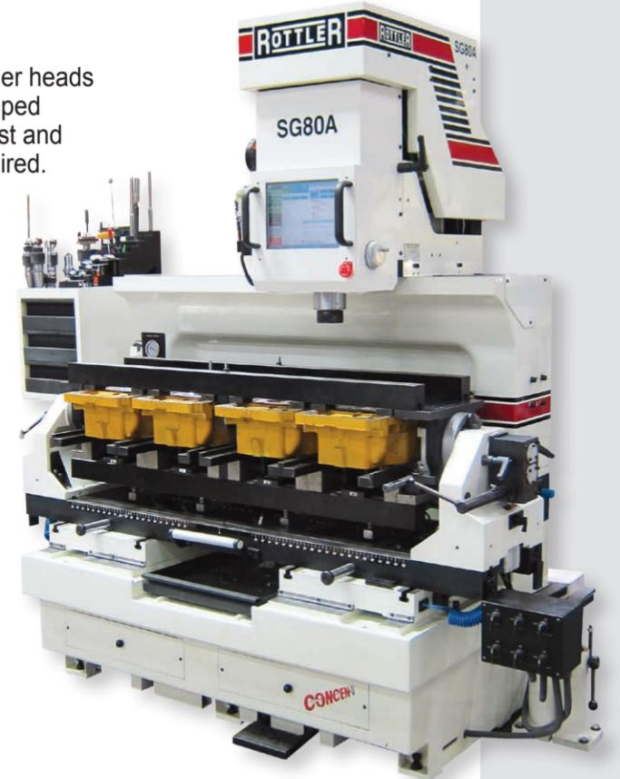
All 24 valve seats, counterbores, and guides can be machined in one set up. Fixture can be rolled 360 degrees for diesel injector and valve spring seat work. Difficult jobs like drilling broken bolts and tapping threads on side of cylinder head can be also done in same set up.
