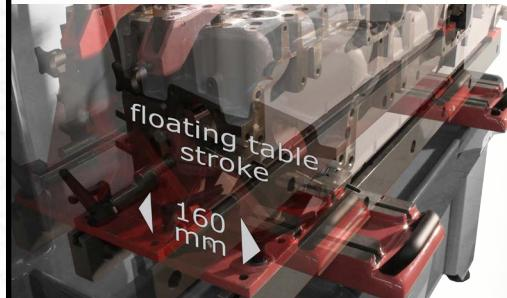
Cylinder heads up to 350 kgs can be moved back and forth without any effort and then locked by two powerful pneumatic jacks.
