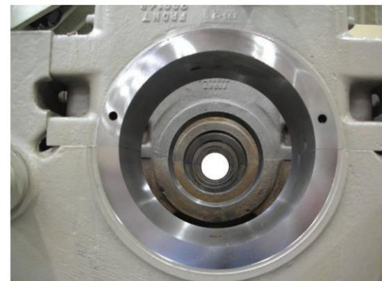
The EM100 series are able to machine main bearing cap registers in the block to ensure they are perfectly flat for maximum contact with main bearing caps. At the same time, the diameter is reduced for line boring back to standard diameter.
